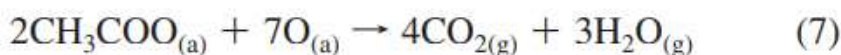
Figure 2 (Partial) ethanol oxidation as proposed by Liu et al., whereas (a) marks adsorbed species and (g) species in gas phase. [30]
