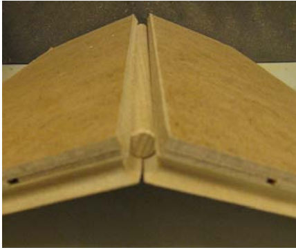
Figure 94: Connection between pieces in the deformed position
