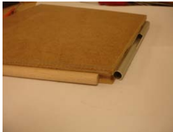
Figure 102: Hole made in some of the metallic cylinders to allow the exit of the cables placed in the ring direction
