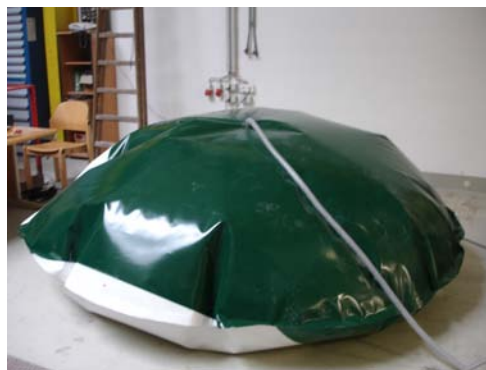
Figure 96, 97 and 98: Pneumatic formwork from the initial plane position to the inflated final one
