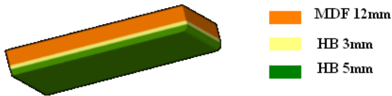
Figure 46: Sketch of the layers of each independent element
