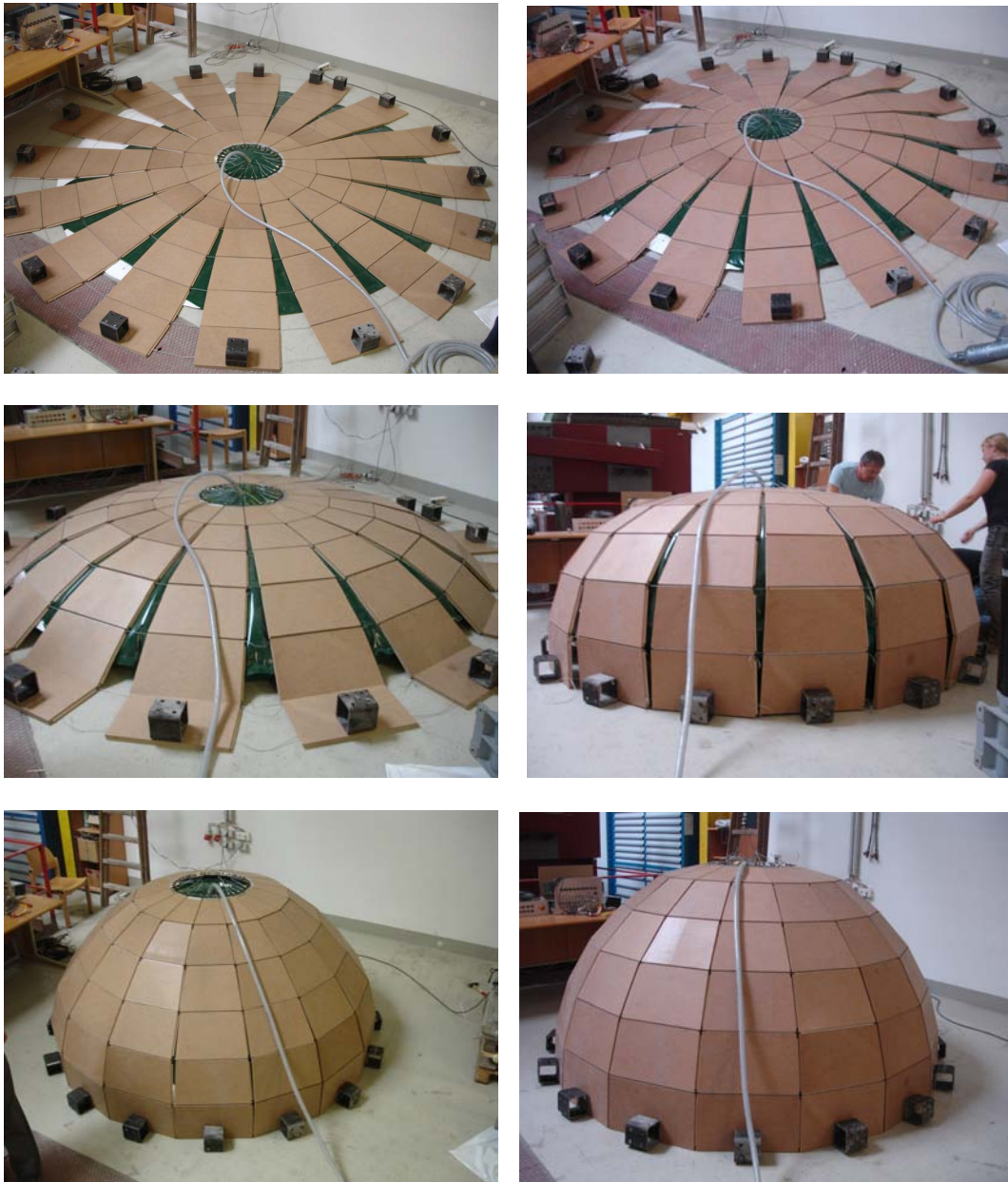
Figure 107: Raising process of the shell
