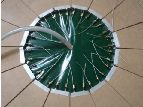
Figure 104: Central ring with all the meridional anchorages
