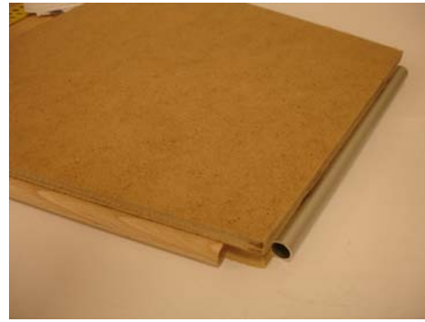
Figure 95: Wood and metallic rods placed on each element
