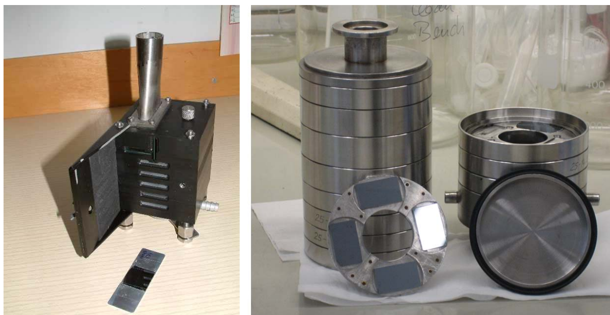
Figure 5.1: Left: 7-stage May cascade impactor and sample collection plate with 20 \times 20 \text{ mm}^2 silicon wafer. Right: Low pressure Berner impactor with a modified impaction plate carrying four Si-wafer plates which were directly used as sample carrier in SR-TXRF analysis.
