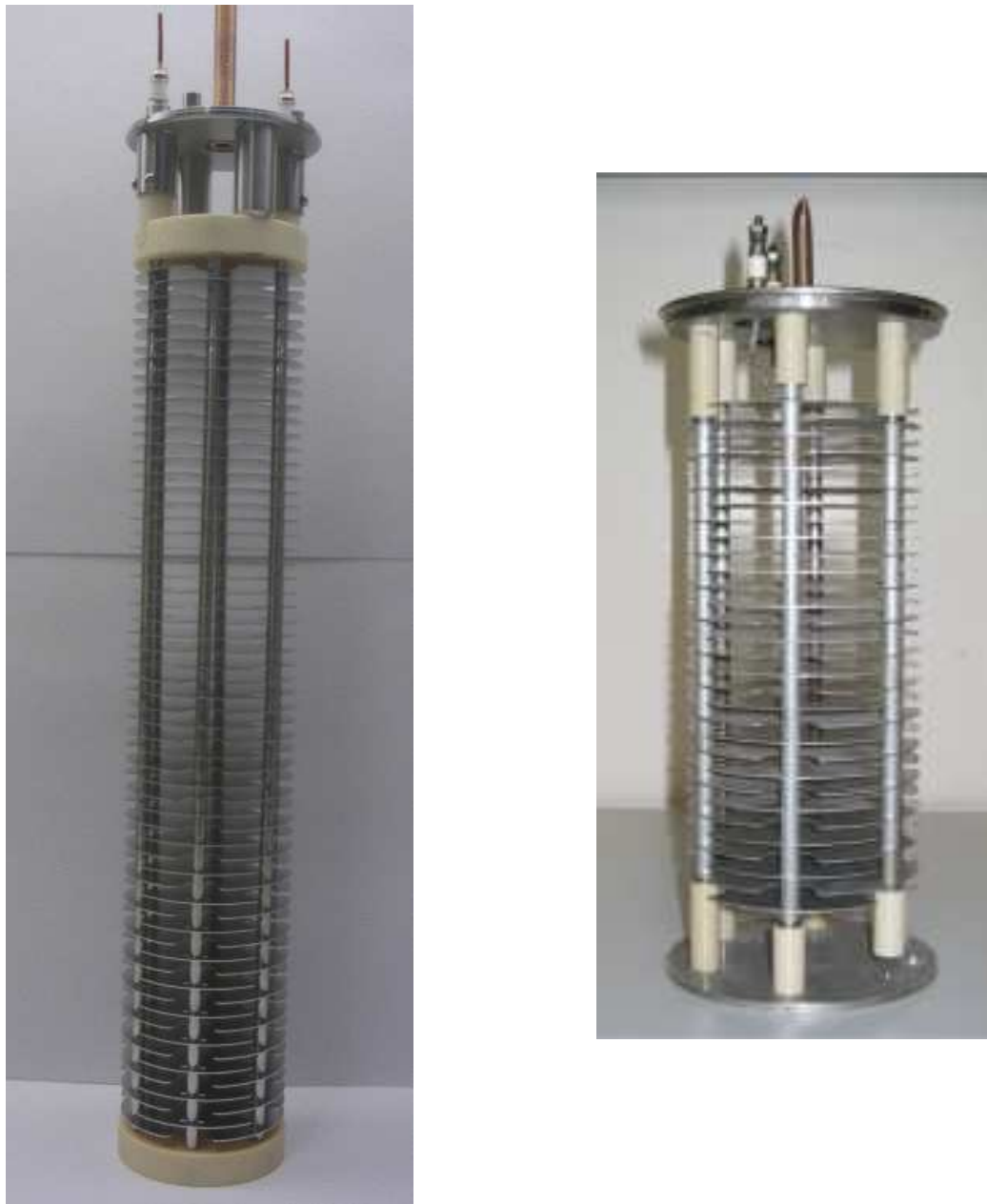
Figure 2.2: Picture of the LHC and the SPS BLM detectors without the cover tube. Left: LHC BLM detector. Right: SPS BLM detector.
