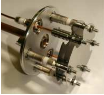
Figure 2.3: Picture of the LHC BLM SEM detector without the cover tube.
