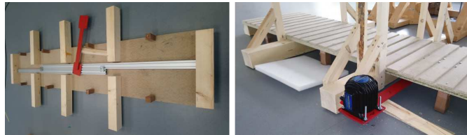
Figure 4.2: Left: Audio transducer mount on the flat bridge prop; Right: underside of the walkway with aluminum rail; Right: audio transducer mounted on metal arm.
