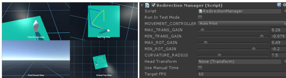
Figure 2.5: Illustration of the built-in capabilities of the Redirected Walking Toolkit for Unity from Azmandian et al. [64]: Views and visualizations (left), inspector configuration parameters for the redirection (right). Configurable parameters include upper and lower bounds for translation and rotation gains, radius for calculating curvature gain and custom head transform object reference.
