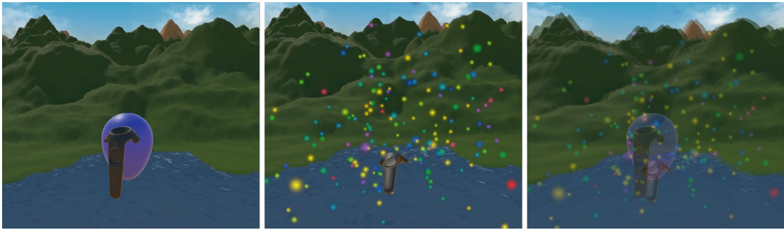
Figure 4.11: Demonstration of redirection introduced during balloon pop. Left: Balloon intact; Center: balloon popped, confetti effect; Right: the two frames overlaid to visualize the rotation introduced at the moment when a user touches a balloon.
