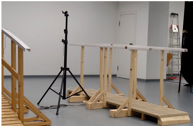
Figure 4.16: Tripod with Vive tracker used to fix floor height in SteamVR.
