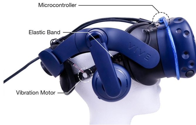
Figure 2.3: Illustration of vestibular stimulator prototype from Peng et al. [56]. They report the best results with the depicted 2-sided vibrator placement setup.
