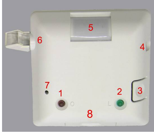
Figure 2.2-5 IT-200, occupancy/state of light (on/off) sensor
