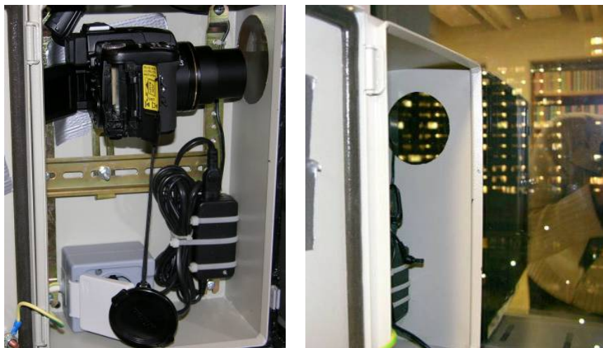
Figure 2.2-8 Camera box with power supply pointing to the VN façade
