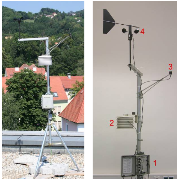
Figure 2.2-1 Left) Weather station mounted on the roof of HB building, right) 1: data logger, 2: temperature/RH sensor, 3: Solar radiation sensor, 4: Wind speed sensor
