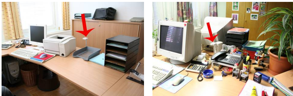
Figure 2.2-4 Position of the Hobo sensors in the offices in HB (left): a single occupancy office, right): a double occupancy office
