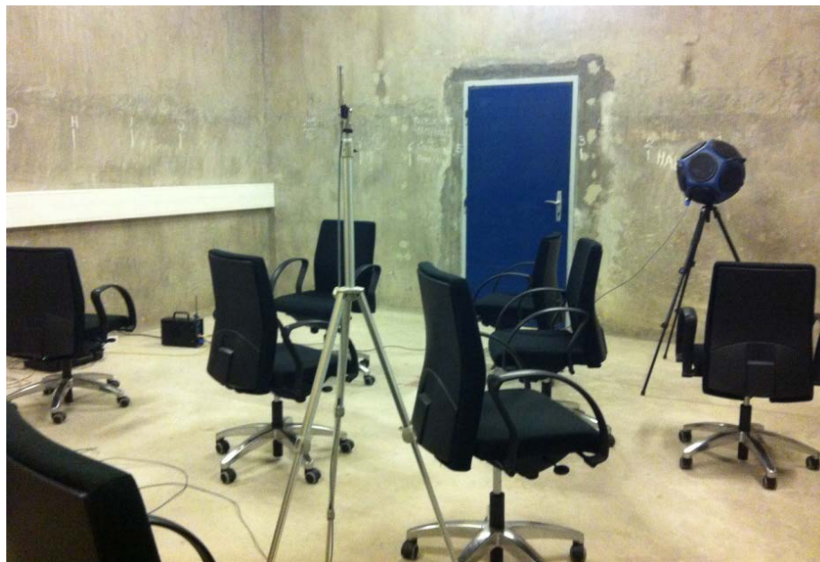
Figure 19 Absorption coefficient measurements of office seats in reverberation chamber
