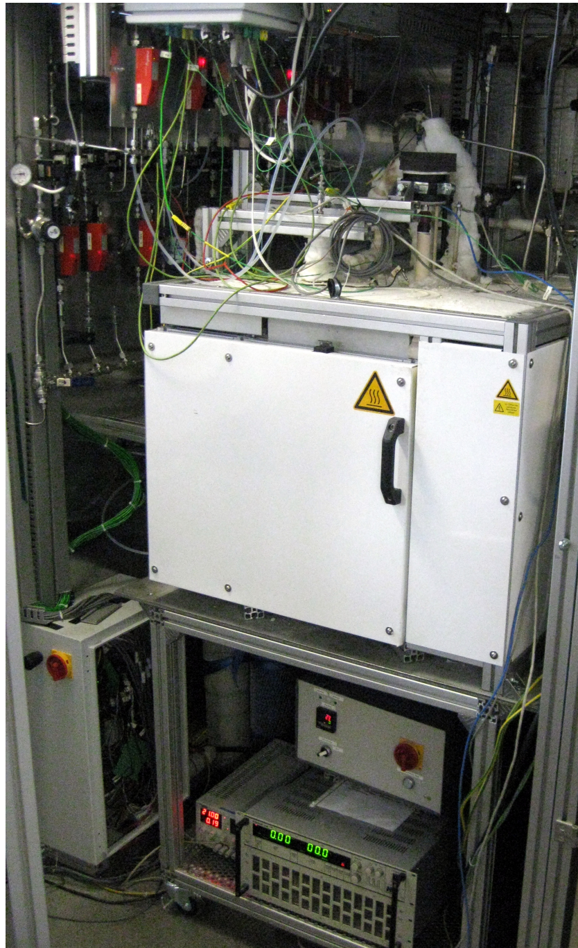
Figure 5.4: Test stand; including furnace, underneath the furnace controller, the electronic load (green digits) and a power supply for SOEC operation (red digits) at the bottom, a electrical control box at the lower left (opened), the gas supply system at the upper left and T-sensors, electric wires and the anode weight above the oven
