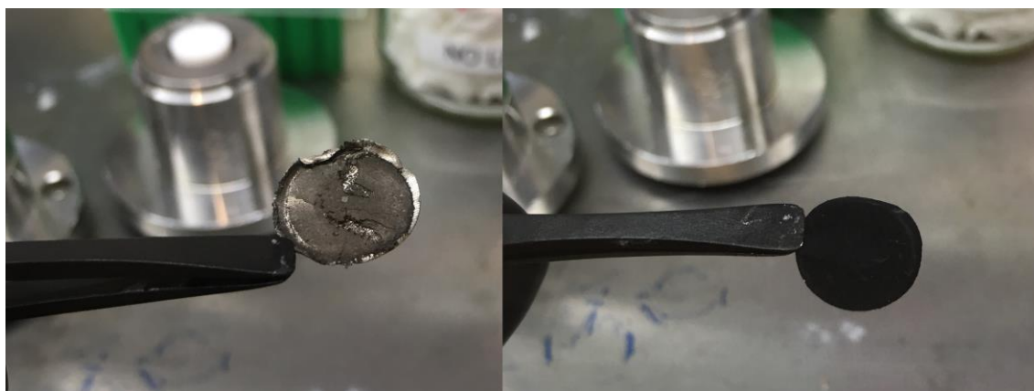
Figure 39. Cathodes from opened and tested cells, cycled (left) and uncycled (right).
