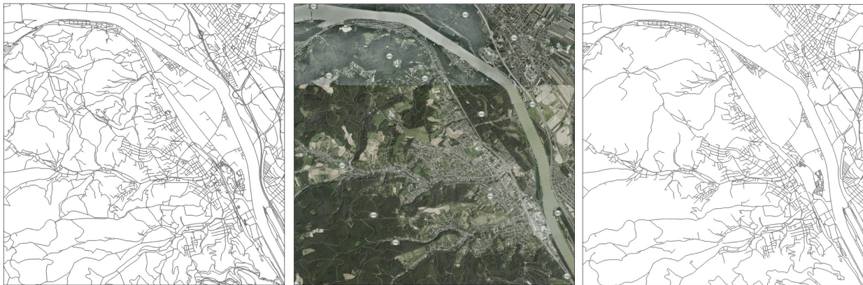
Figure 33: Development of the network layer (right) based on OpenStreetMap street data (left, Karch and Ramm 2012) and Orthophoto (middle, Geoimage 2011)
