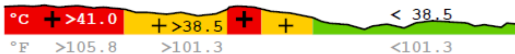
Figure 3.47: Qualitative - quantitative hybrid as used in Midgaard. The quantitative data of a fever curve is represented by the height while additional qualitative information is provided by the color-coding (critical fever values are colored red, moderate fever yellow and normal temperature green) [10].
