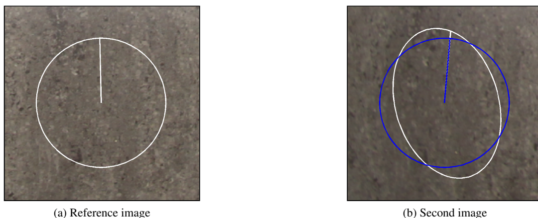
Figure 4.7: Original SIFT feature detected in reference image and its transformed illustration in second image (white). Estimated SIFT feature in second image with adapted scale (blue).
