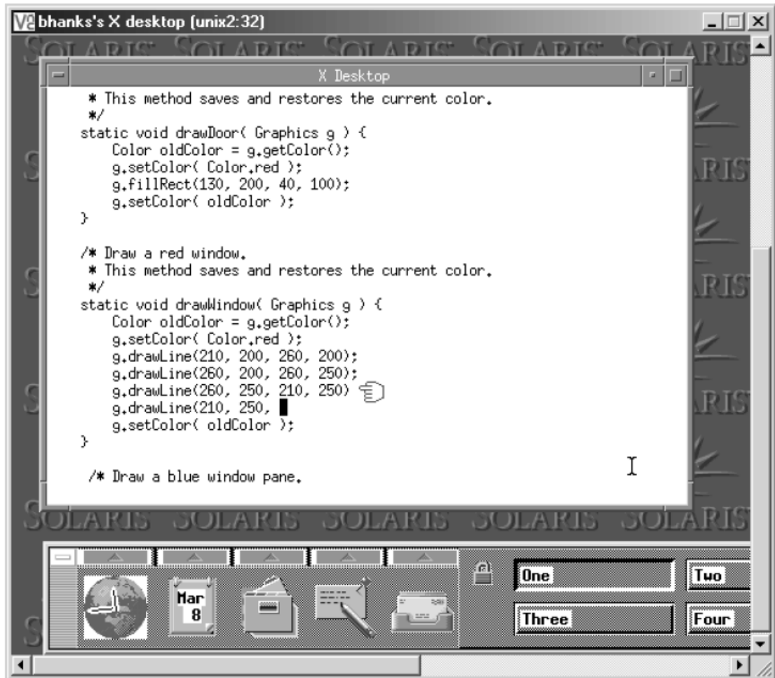
Figure 11. Gesturing mode of the VNC Extension for Distributed Pair Programming [Hanks, December 2005]
