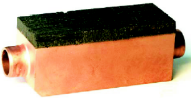
Figure 1.4: Image of the flat tile mock-up design.
