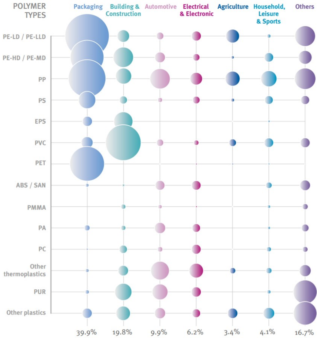
Figure 2.3: Plastics demand by segments and polymer types in 2018 data for EU28+NO/CH (51.2Mt) [64]
