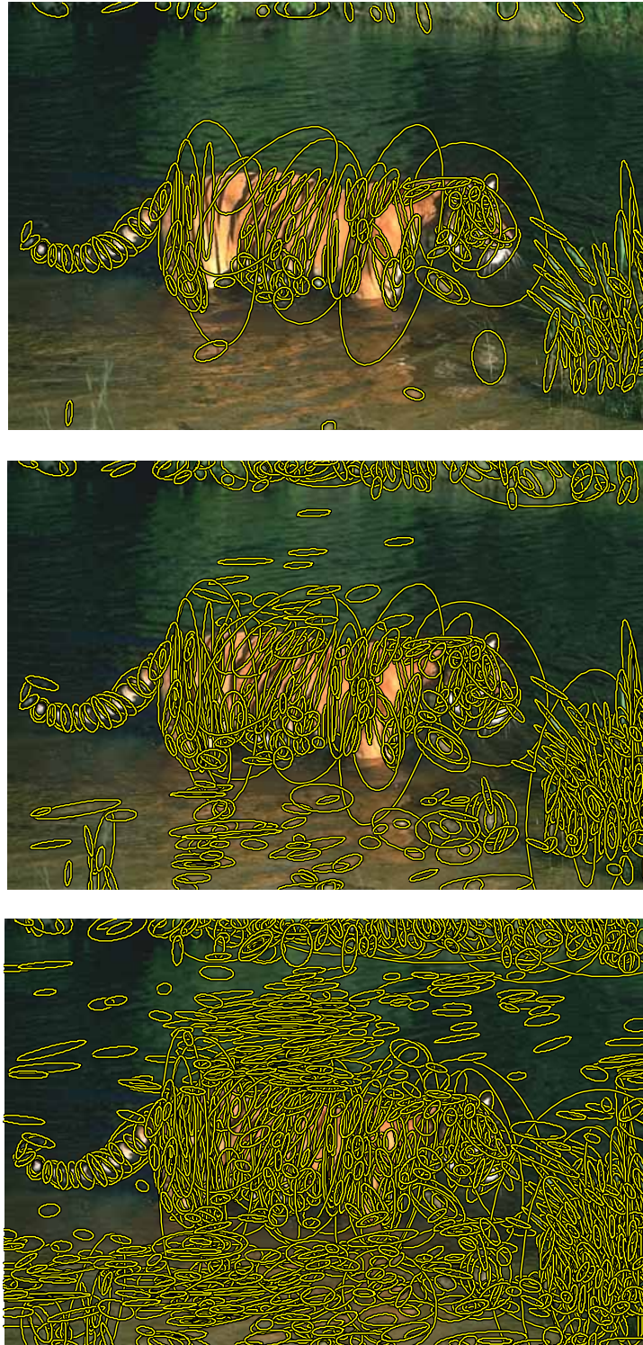
Figure 2.11: The result of MSER region detection with varying parameter M . From top to bottom M = 20, 10, 5 . MSER regions are represented by fitted ellipses.
