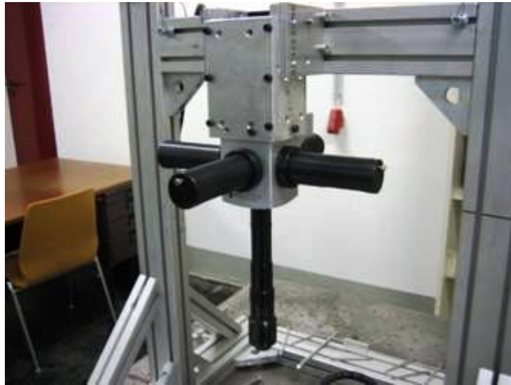
Figure 6.2: Electronic speckle pattern interferometry (ESPI) [18]
