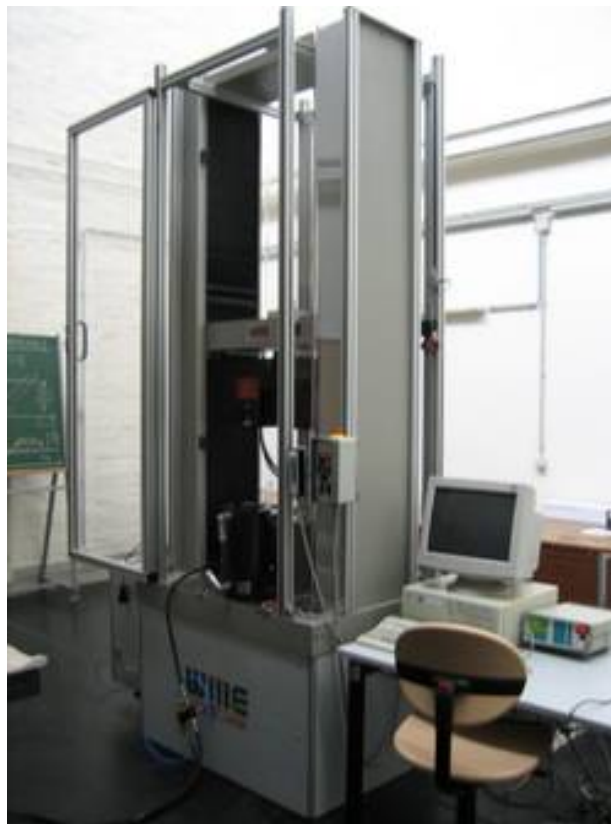
Figure 6.1: Uniaxial electro-mechanic universal testing machine (UNIAX) [18]
