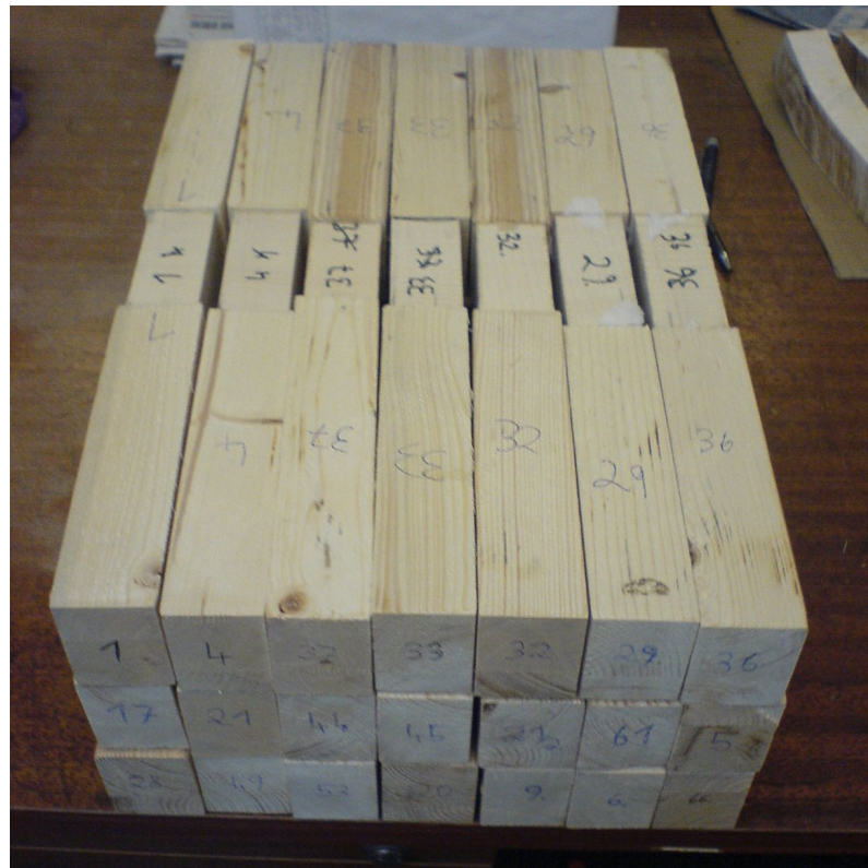
Figure 6.7: Blank shape of the glued samples from BOKU
