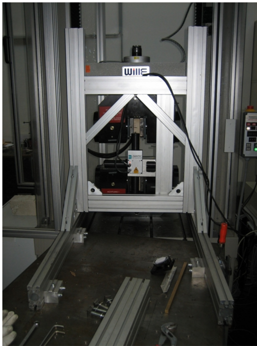
a) ESPI-system fixed on a moveable heavy desk in front of the tension testing machine
