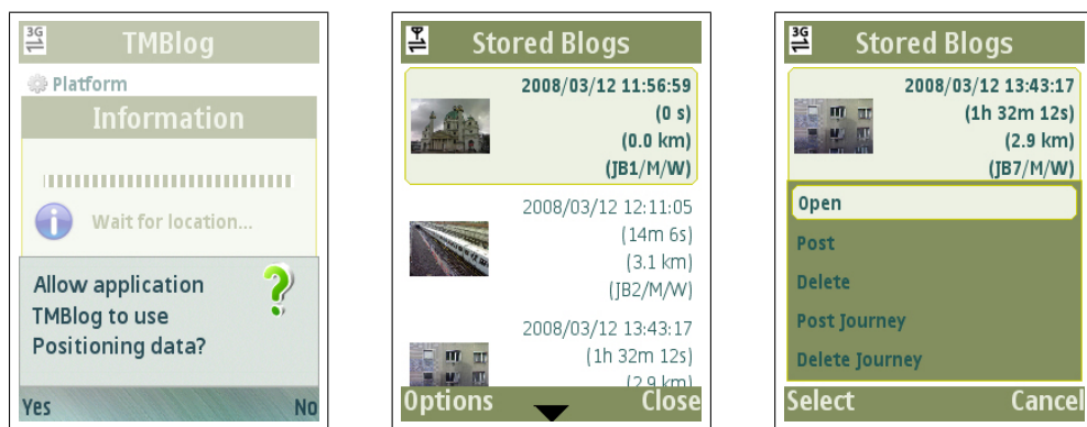
Figure 6.9.: Screenshots of the Mobile Client - The System's Security-related Capability Feature confirms the User during the Location Determination Process since the Application is not Signed (left). Exploration of stored Waypoint-related Journey Blogs. The List Items represent generated Blogs and refer to their Content as well as to their spatial and temporal Relationship among each other (center). Several Operation can be performed on stored Blogs (right)
