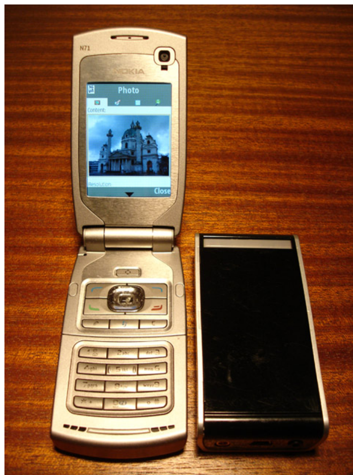
Figure 6.12.: A Nokia N71 handset has been used in the Prototype Testing Phase. An external GNS 5843 Bluetooth GPS Receiver enabled an accurate Determination of the User's geodetic Location.
