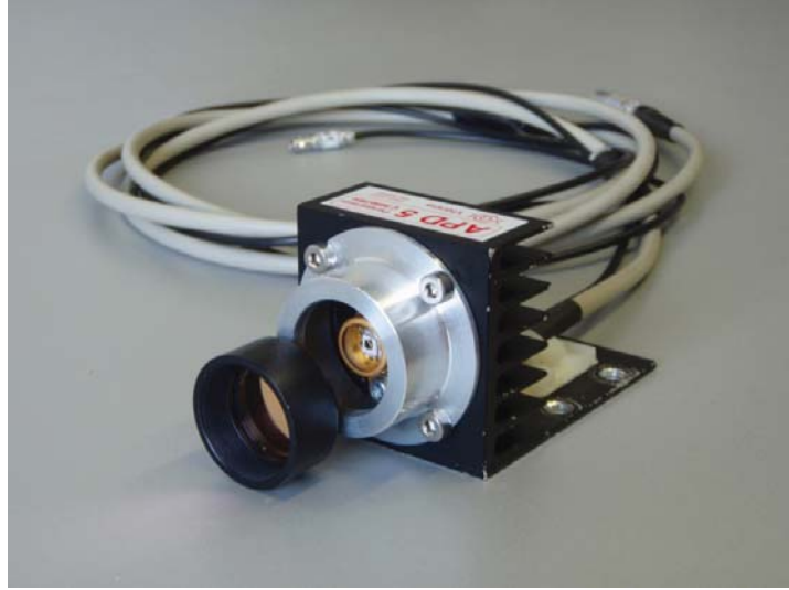
Figure 3.6: Our passively quenched single-photon detector and the bandpass interference filter.
