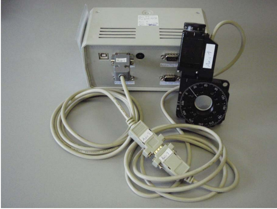
Figure 3.5: The Standa 8MR150 motorized rotation stage and its controller 8SMC1-USBh-B2-4PS .
