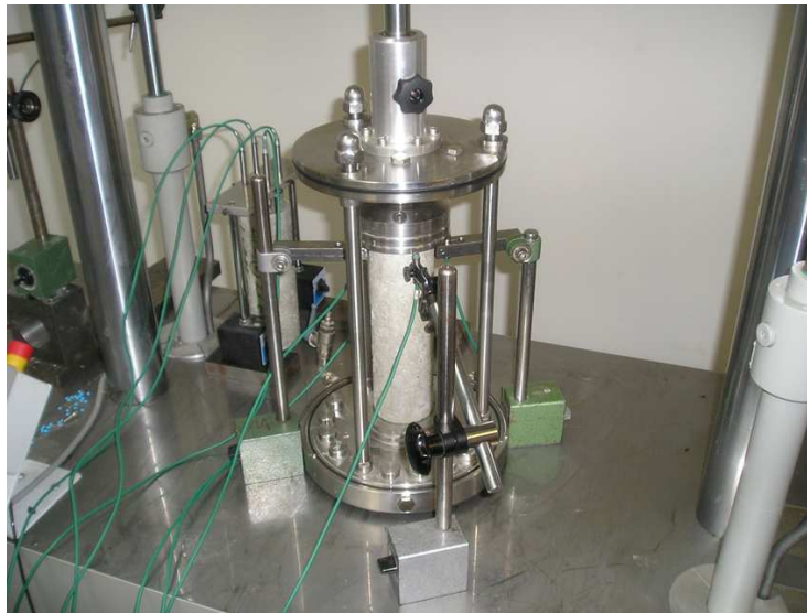
Figure 3.1: Test arrangement for uniaxial testing of shotcrete
