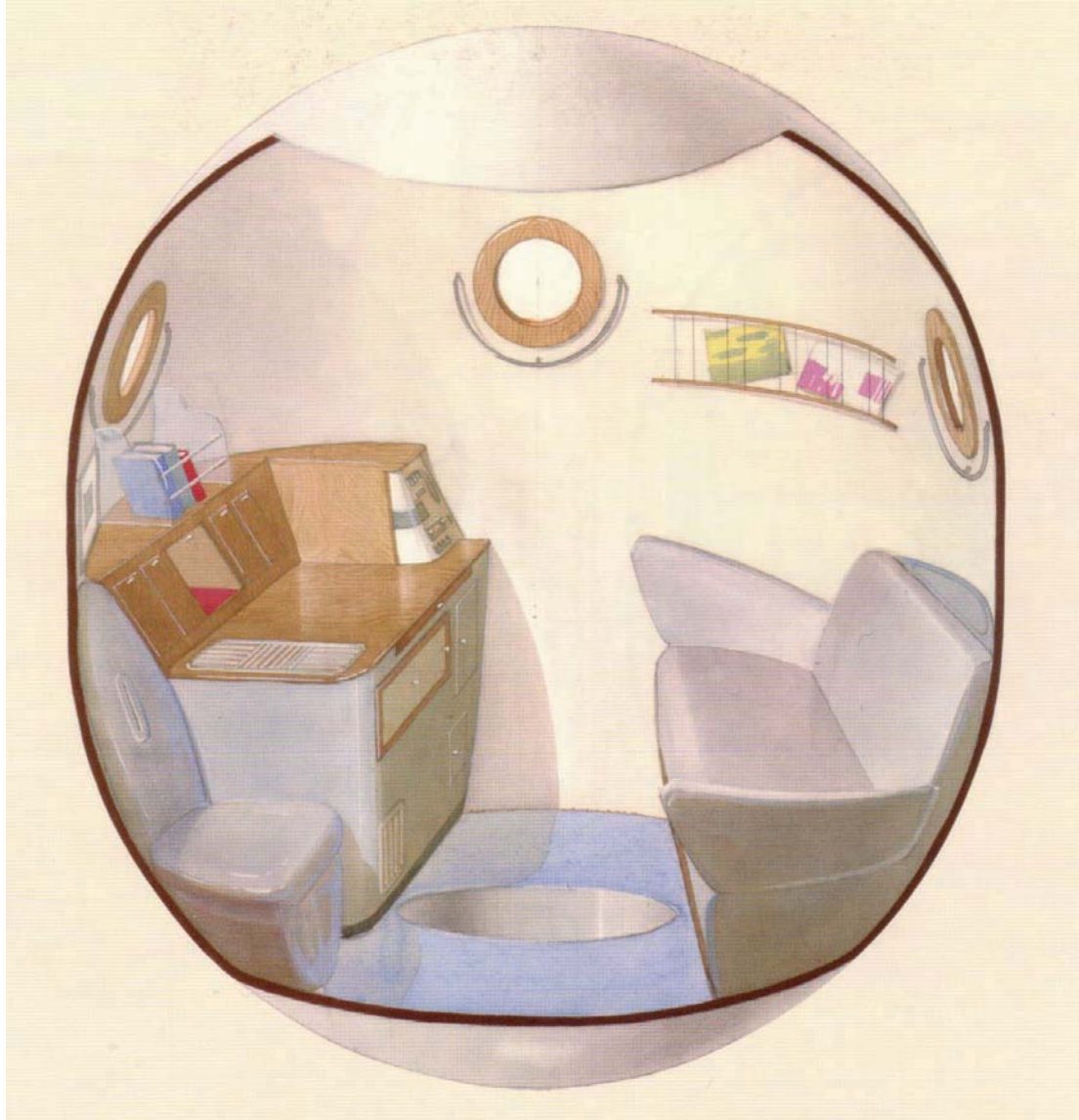
Figure 1-12: A sketch showing one of the earliest considerations for the interior of a Soyuz orbital module with a living room atmosphere, which was never created that way. The conventional references are likely to fail in extreme environments. (Credit:RKK Energia)
