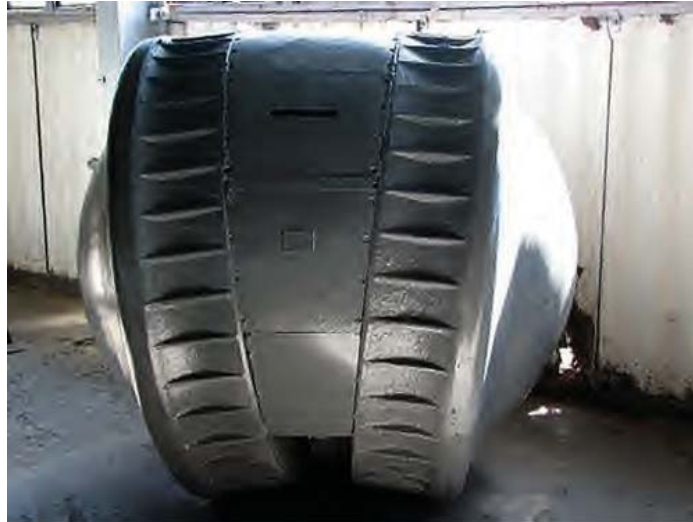
Figure 3-29: Krupp Kugelpanzer prototype. This diwheel one-man armored vehicle was designed to operate under extreme conditions of battleground environment. (Source: www.jagdtiger.de )
