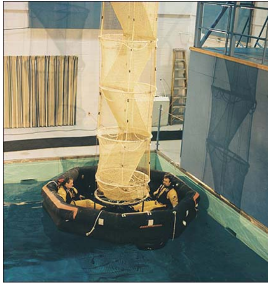
Figure 1-7: The Hibernia Oil Platform can be evacuated via escape chute / raft systems in an emergency case. Escape chutes have to be used in combination with surface rescue units. (Source: CHHC)
