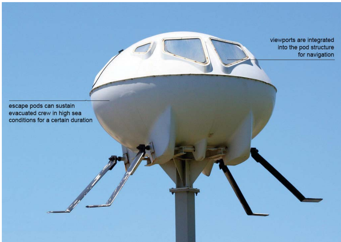
Figure 1-6: An escape pod mounted on an oil platform. Escape pods resemble advanced lifeboat type self-rescue measures (Raw image source: Flickr, Edit: Özdemir)
