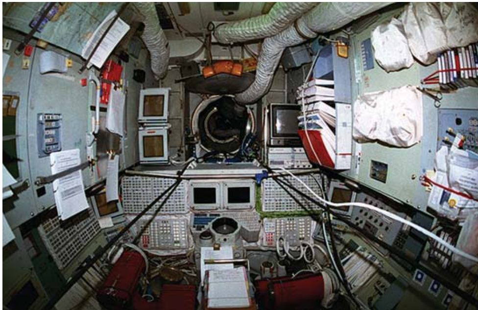
Figure 3-24: An image from the interior of the retired Mir space station. Note the improvised connection lines between the modules 24 (Credit: NASA)
