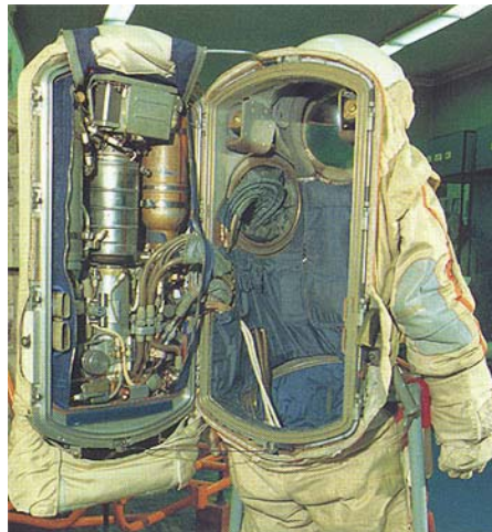
Figure 3-73: A rear-entry Orlan-DM space suit. Note the backpack-integrated life support system (Credit: NPP Zvezda)
