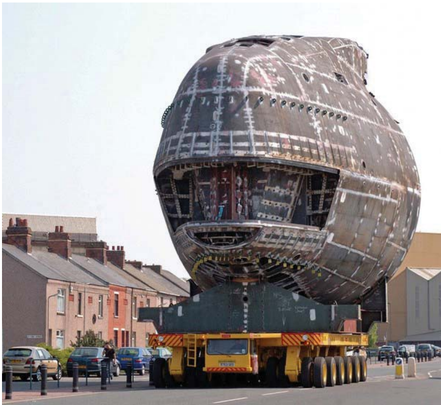
Figure 4-2: The bow segment of a nuclear submarine during transport to assembly facility through the streets of a small town. We need accessible and relevant design knowledge rather than common or garden architectural design references. Space is an extreme environment! (Credit: Getty Images)
