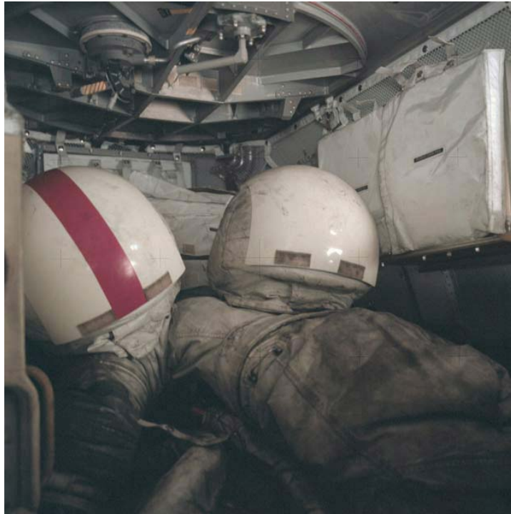
Figure 3-67: Dusty gear of the Apollo 17 astronauts stowed in the Lunar Module after an EVA. Dust poses a serious problem to all lunar habitats. (Credit: NASA)
