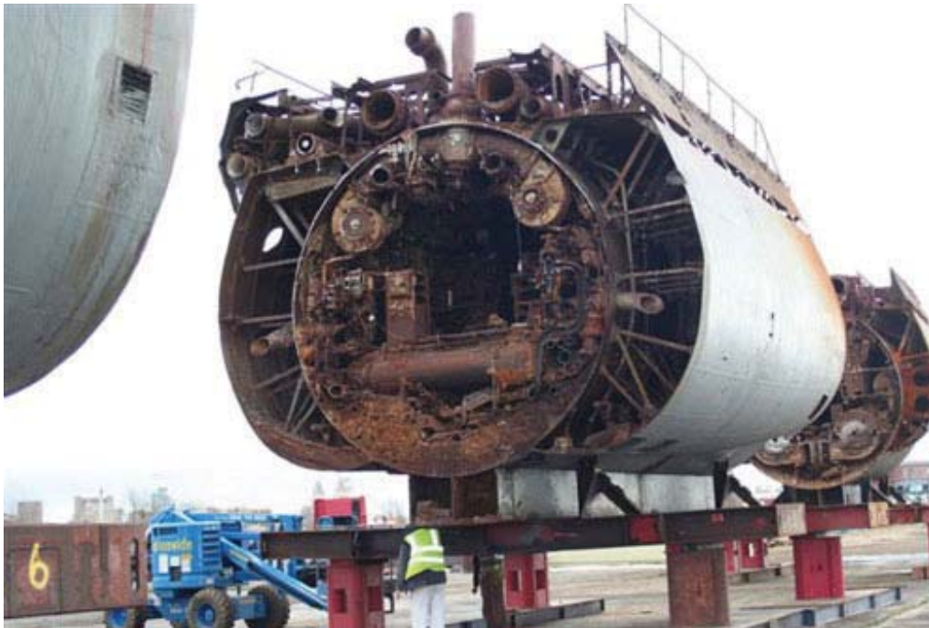
Figure 3-41: The section of the salvaged U-boat U 534. All the habitable spaces of a submarine are housed inside the cylindrical pressure hull. Analogous to space habitats, the pressurized vessel is equipped with a network of utility systems. (Credit: Barr)
