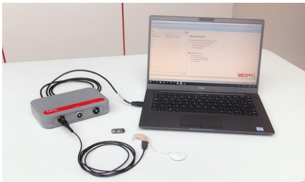
Figure 1.2: MED-EL cochlear implant fitting setup
