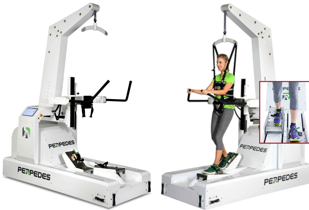
Figure 4.1: Schepp Medtech's PerPedes [Med15]. Robotic gait rehabilitation with plantar flexion and dorsiflexion support. The system provides vertical GRF readings for both feet. Since the subject's feet are strapped in (red frame), negative forces can potentially occur. Images taken from the manufacturer [Med15] and the SFG [Ste17].
