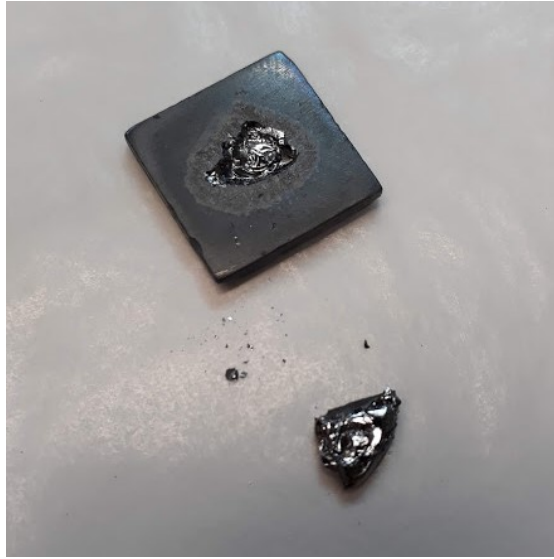
Figure 4.16: Picture of the reacted sample holder and the destroyed sample after the measurement. Obviously a melting process took place.
