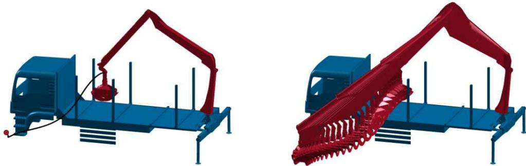
Figure 4.17: Resulting state trajectory of the simulated, augmented Lagrangian based MPC-controlled crane.
