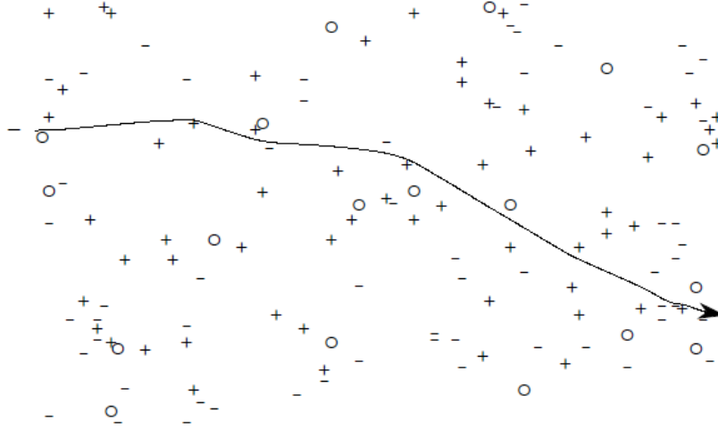
Figure 2.21: Schematic of a test particle trajectory in a plasma with electrons (-), positive ions (+) and neutral (circles). The trajectory will be altered as a consequence of many, small angle Coulomb collisions. [53]
