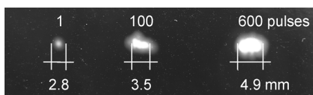
Fig. 36: Focused beam profiles at 40 m with varying pulse numbers per spot; increasing pulse accumulation shows the point stability which is limited by atmospheric fluctuations
