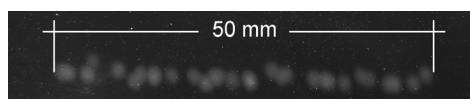
Fig. 38: Line scan of focused laser spots on photo paper at 40 m distance; achieved with motorised mirror mount; average distance between consecutive burn spots is 1.75 mm
