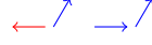
Figure A.2: The eigenmodes of two dipoles on a hexagonal grid. The arrows show the direction of carrier movement, while the color indicate the sign relative to the base vectors. Red stands for an oscillation, which is anti-parallel to the base vector.
