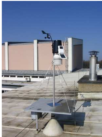
Figure 6.1: Weather station on the roof of the Institute
