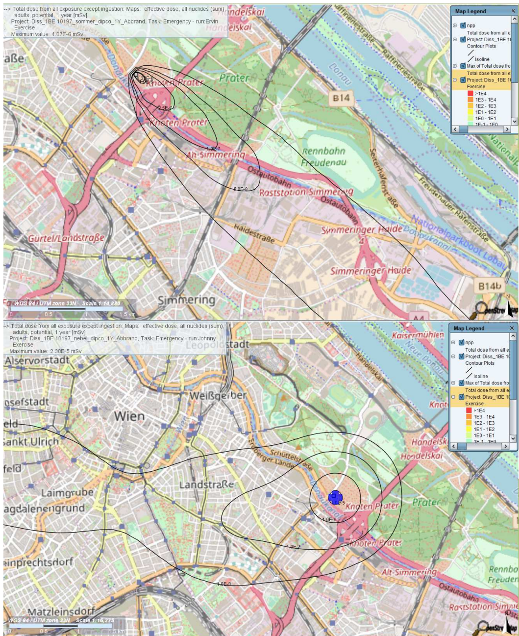
Figure 8.1: Comparison of the summer (top) and foggy day scenario (bottom), effective dose after 1 year, exposure of 1 fuel element, 1 year of burnup
