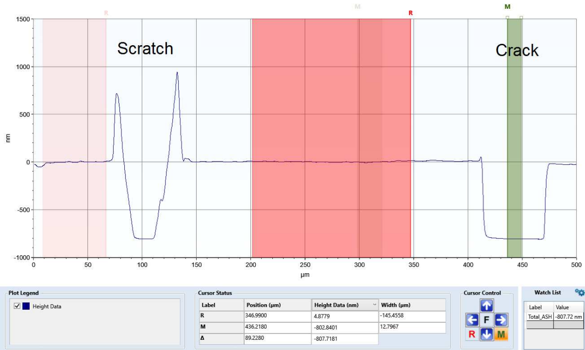
Figure 21: Example of a profilometry measurement showing a scratch and a crack
