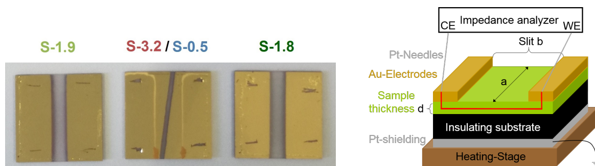
Figure 56: Samples for the in-plane measurements (S-0.5 was produced using S-3.2)
