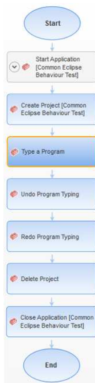
Figure A.6: UFT flow diagram for guideline 3.5/10 "UNDO to Reverse Control Actions"
