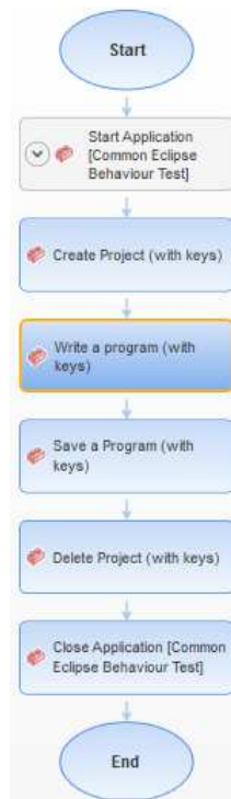
Figure A.4: UFT flow diagram for guideline 3.1.3/7 "Menu Selection by Keyed Entry"
