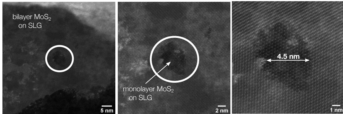
Figure 7.10: Regimes of present bilayer MoS 2 on top of SLG as a result of CVD growth. Ion-induced pores by irradiation with 166 keV Xe 38+ ions only in the first layer of MoS 2 . The second layer as well as SLG beneath the pore stay intact.
