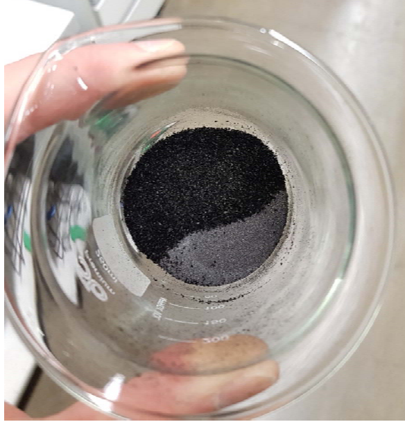
Figure 90: Filter content after five cycles, using ilmenite as OC and wood pellets as fuel
