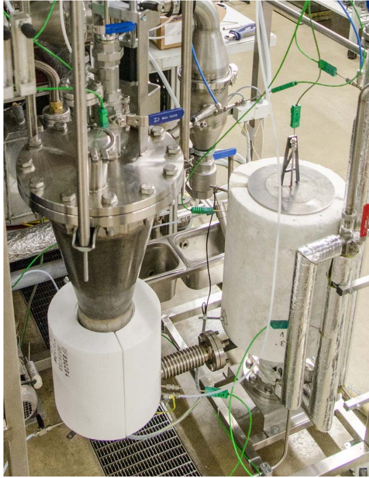
Figure 63: Preheater and reactor in detail before insulating
