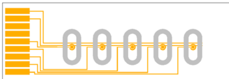
Figure 3.6: Sensor layout with measurement chambers for each working electrode
