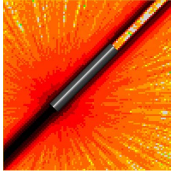
Figure 26: Fluence per primary particle of all particles showing the widening of the 250 MeV proton beam when it hits the target with 5 cm diameter
