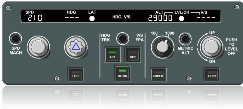
Abbildung 17: Flight Control Unit (FCU). (Quelle: CBT Honeywell International Inc., Deutsche Lufthansa AG)
