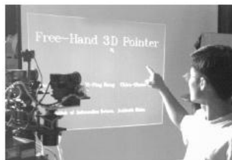
Figure 2. This figure illustrates the operation of our free-hand pointer. The speaker is pointing his index finger to the projection screen (under the word "3D"). The IIS head on the left takes the stereo image pairs to be processed. According to the projection site determined from the stereo image pairs, the computer then controls its cursor to the word "3D".
