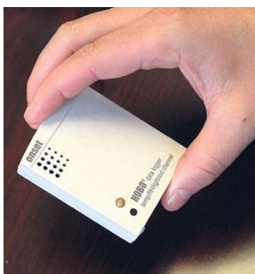
Figure 11: Onset HOBO U12-012 data logger (Arney, Pantagraph, 2008).
