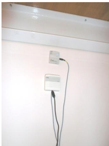
Figure A-18: After School Group 4, CO 2 sensor and wall mounted temperature / humidity logger.
