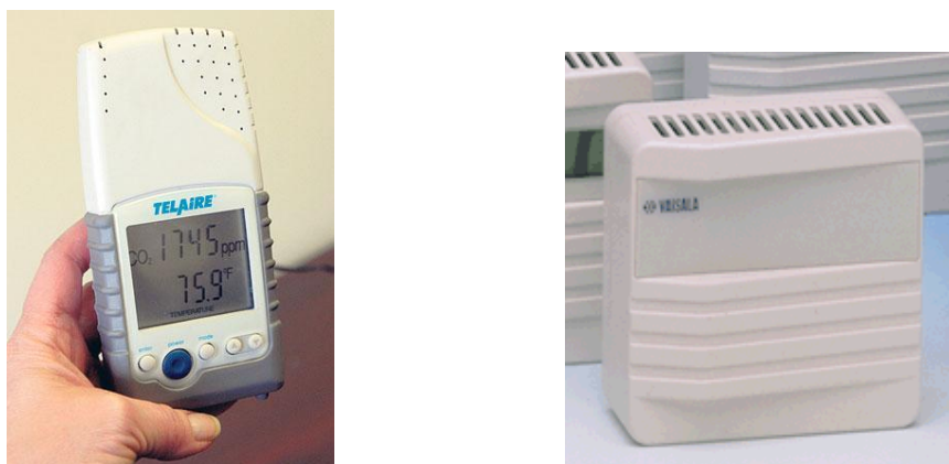
Figure 12: Telaire 7001 and Vaisala Carbocap GMW22 carbon dioxide monitors (Arney, Pantagraph, 2008; Vaisala, 2009).
