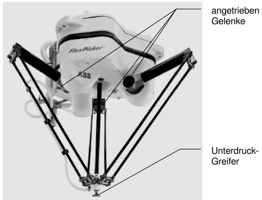
Abbildung 16: ABB-IRB 340, "Pick & Place"-Roboter [33]
