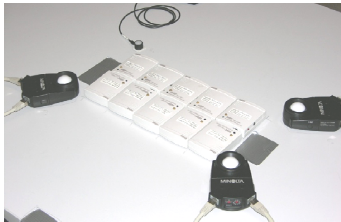
Figure 2-40 Calibration setup for HOBO illuminance sensors
