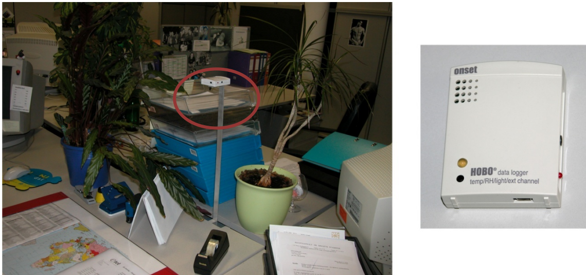
Figure 2-22 HOBO U12-012 logger, mounted at a workplace in ET and close-up
