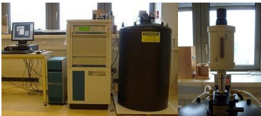
Figure 3.6: Physical properties measurement properties system vibrating sample magnetometer (VSM) PPMS Q6000 (Quantum Design) at TU Wien.
