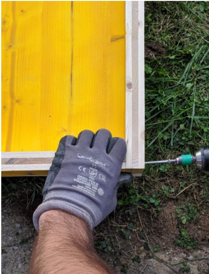
| Creating the casts for the Riverstone Concrete tests
