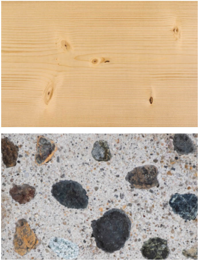
I Exposed aggregate concrete is used for the foundation. The interior is covered with sanded and oiled spruce plywood
