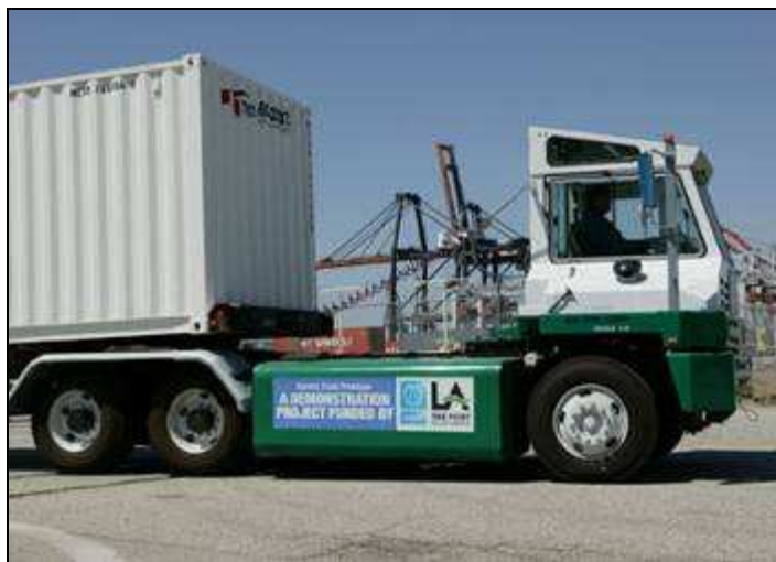
Abb. 5.21 Short-Haul Heavy-Duty Electric Truck Nautilus E-30 am Port of LA; Quelle: [Q 182]
