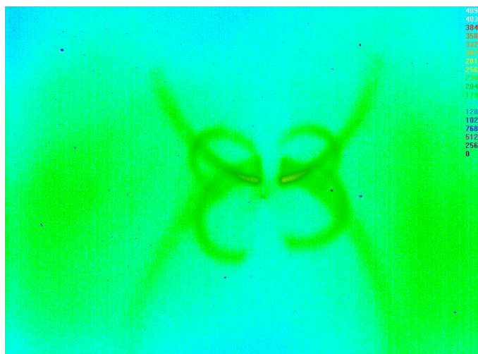
FIGURE 27: Picture of ring system of the full setup. A 6nm bandpass filter was used to select the rings with correct wavelength.
