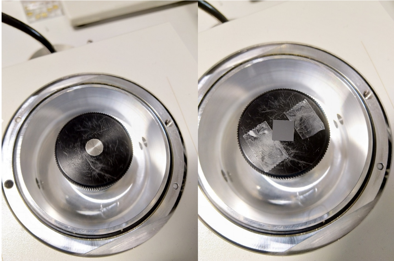
Figure 45: Collector, left: electrode without wafer, right: electrode with silicon wafer attached.
