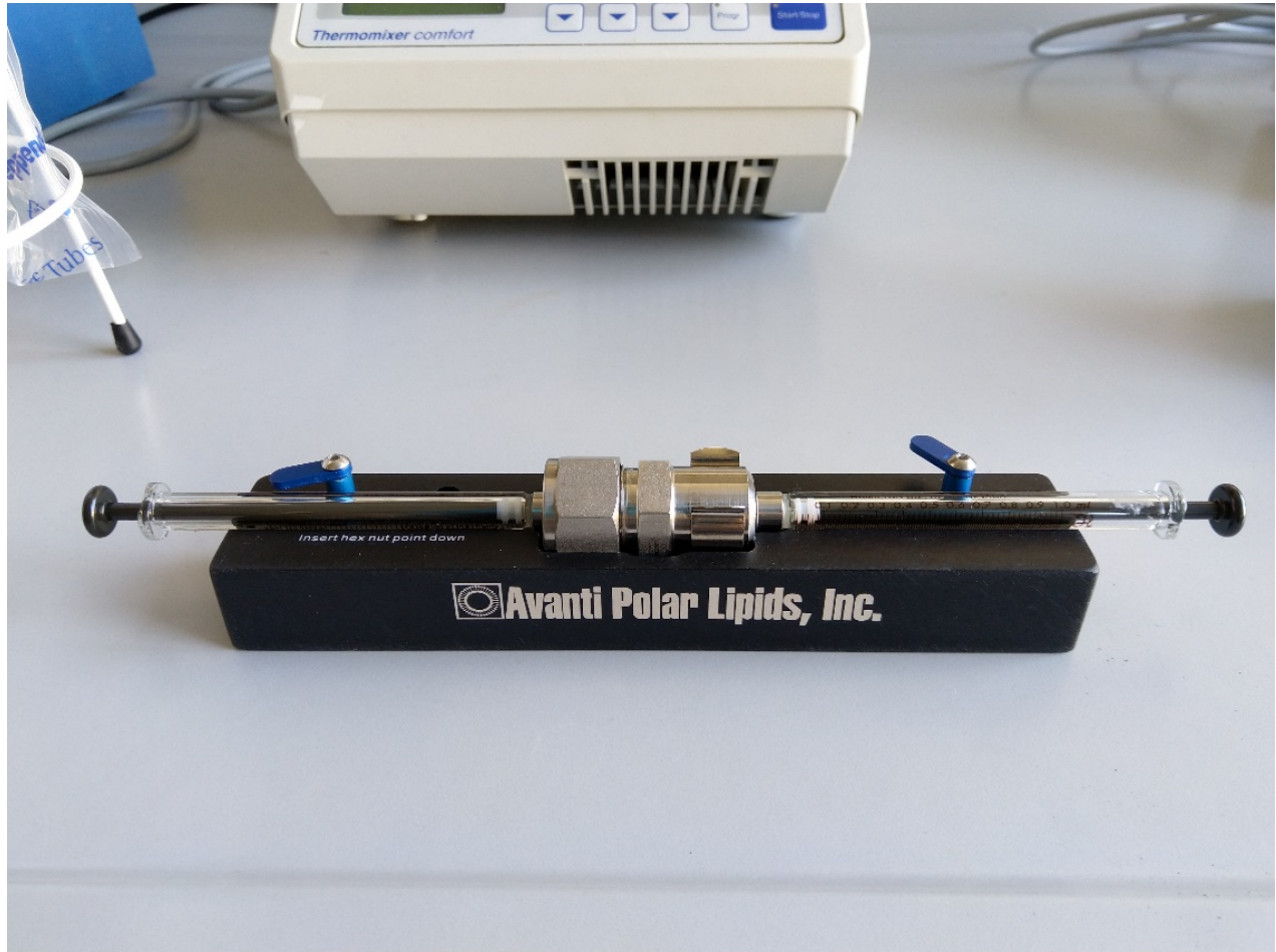
Figure 12: Extruder used to create the liposomes.
