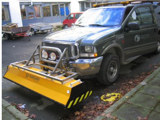
**Abbildung 18: GPR (Ground Penetrating Radar) [13]**
