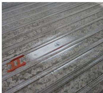
Figure 18: Heat conduction paste is applied onto the surface.
