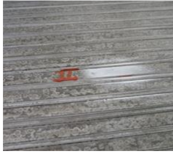
Figure 15: The surface where the temperature sensor is applied, is cleaned.
