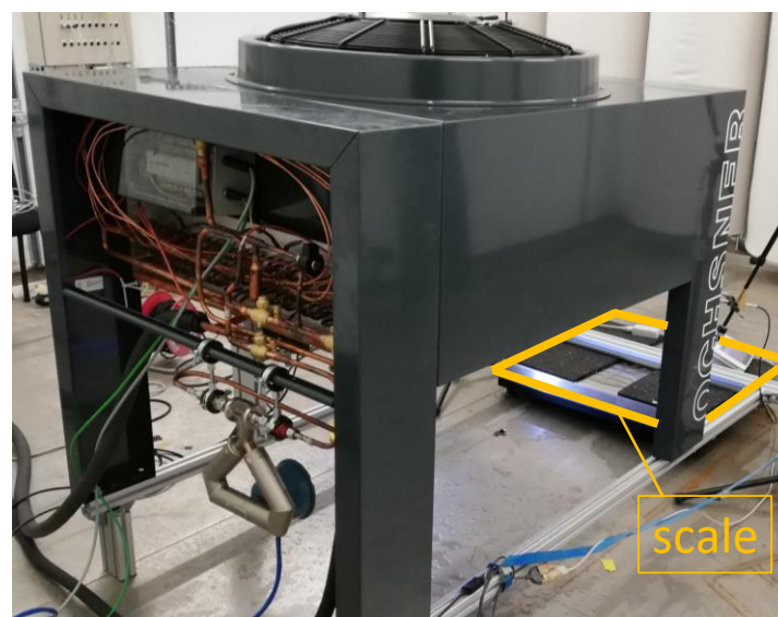
Figure 23: Evaporator inside the climatic chamber is mounted onto a scale to measure changes in weight.
