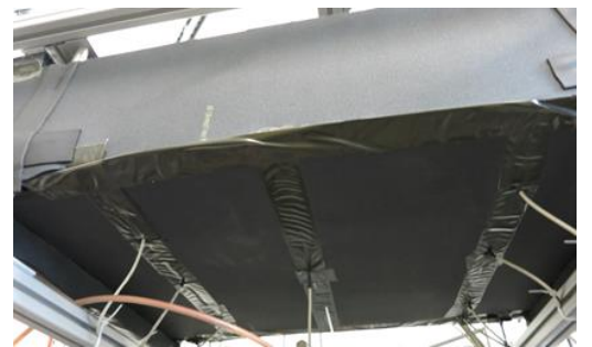
Figure 20: The RPW-HEX is completely insulated, cables from the temperature sensors were routed through the insulation.
