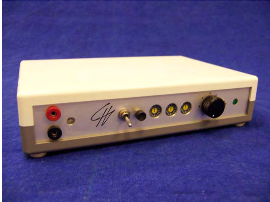
Figure 3.17: Picture showing the front plate of the stimulator with the jacks for the electrode cables, output indicator LED, switch and push-button for triggering the stimulation and activating the continuous mode respectively, binary coded switches for setting the stimulation parameters, potentiometer for setting the output voltage and power on indicator LED (from left to right).
