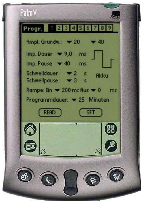
Fig. 3.11: A personal digital assistant showing the graphical user interface for programming the stimulator is shown.
