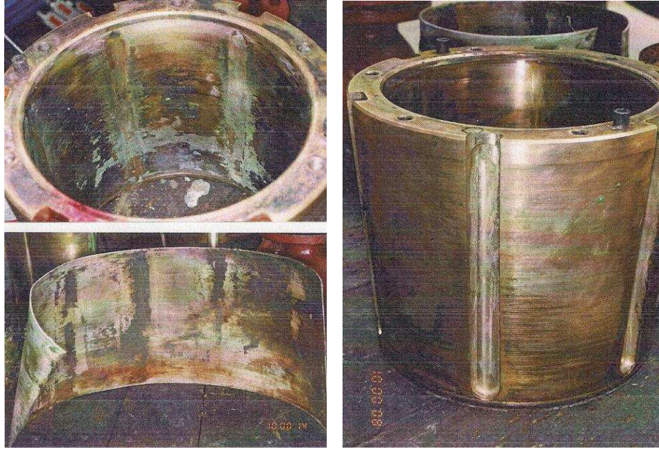
Fig.3. 22: The deformation of bronze bushing [17].
