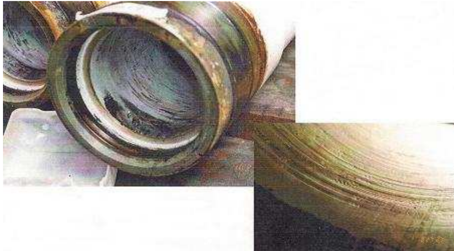
Fig.3. 24: Wear on the Teflon film [17].
