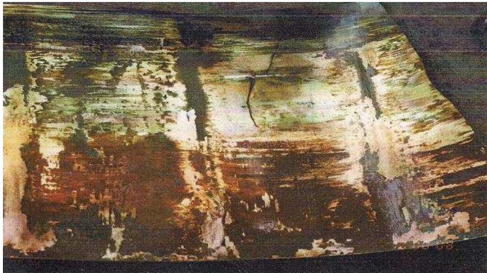
Fig.3. 21: Crack in the Teflon film of the lower bearing [17].
