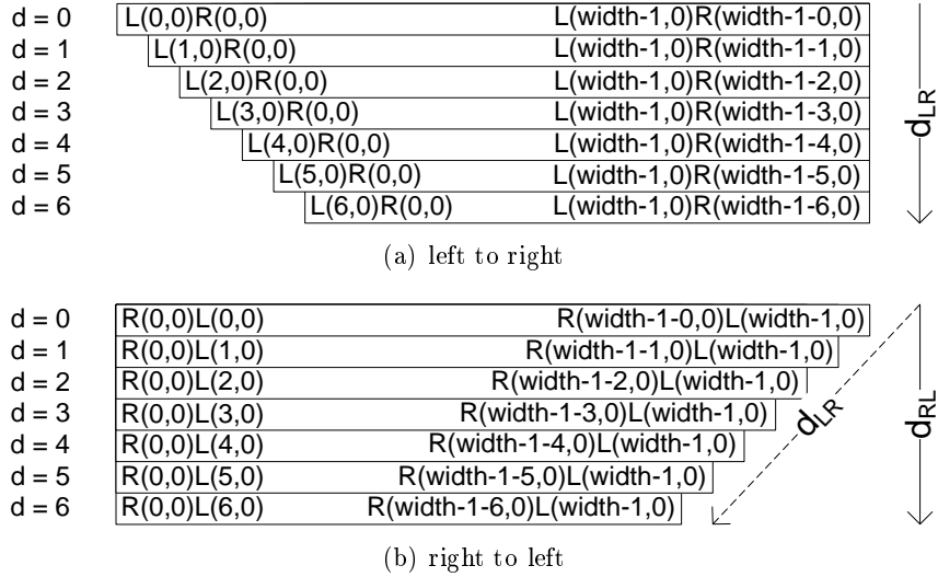
Figure 4.7: Disparity space image entries for one line at 6 disparity levels with the WTA search directions
