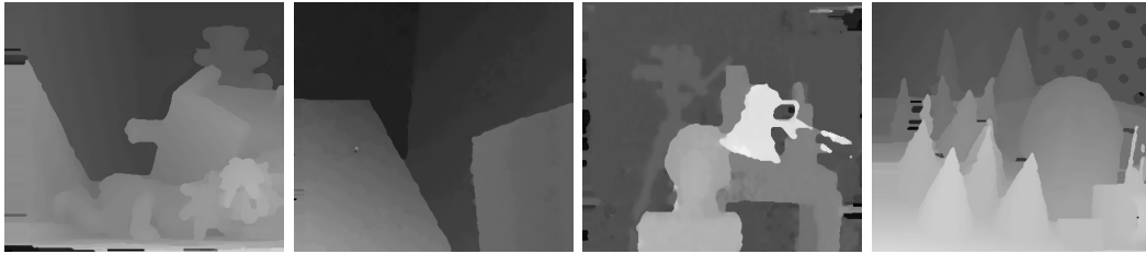
Figure A.4: The results of the proposed algorithm (Census correlation with SGM and color-based segmentation) for the Middlebury datasets.
